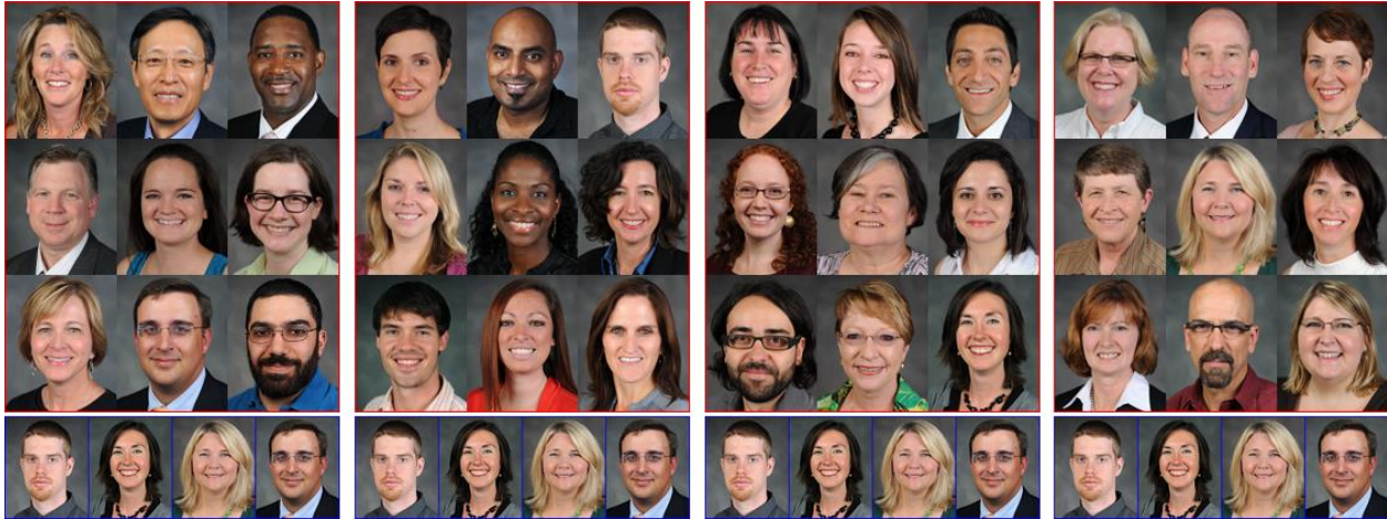
Figure 3: Four consecutive grids of faces (top area) and the password guide (bottom area, repeated) used in PassFaces. Each grid contains one face from the guide that the user must tap to log in.
