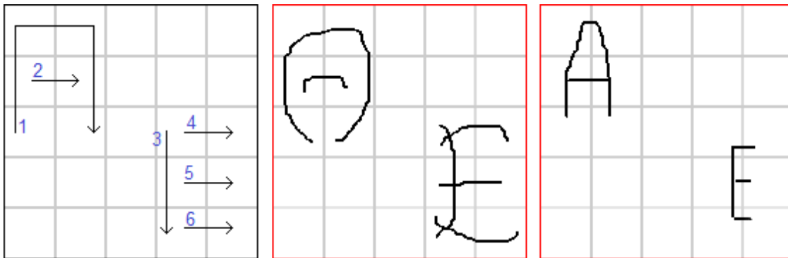
Figure 1: On the left is a guide for a DAS prototype indicating lines to be drawn and the drawing sequence and direction. In the middle and right are two samples that, if drawn in the correct sequence and direction, would successfully authenticate the user.
