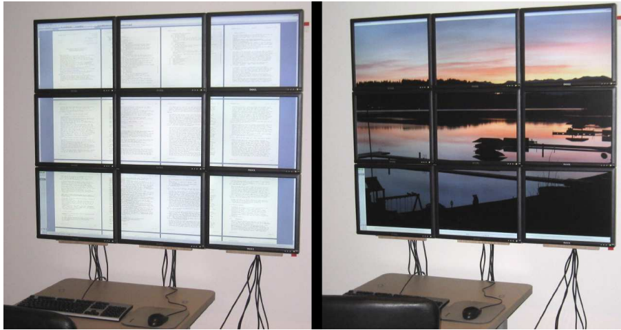
Fig. 2. A computer with nine display monitors configured as one large workspace.
